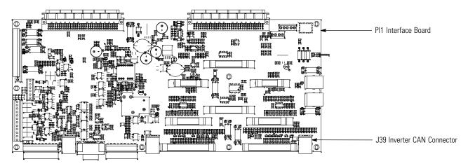
Figure 4-16. J39 Location on PI1 Interface Board
